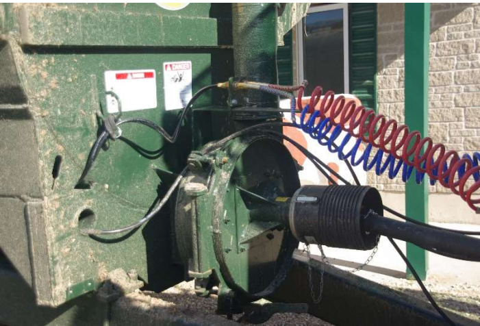
8" discharge up to 3600 gallon per minute adjustable
