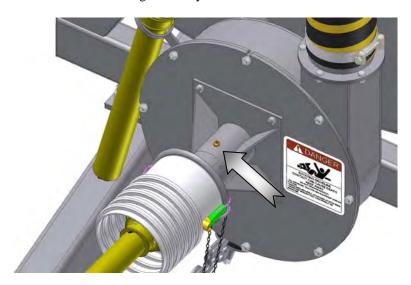
FIG. 7 BEARING ASSEMBLY GREASE
