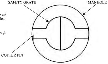
FIG. 5 MANHOLE GRATE
