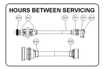
FIG. 5 PTO DRIVELINE SERVICING
